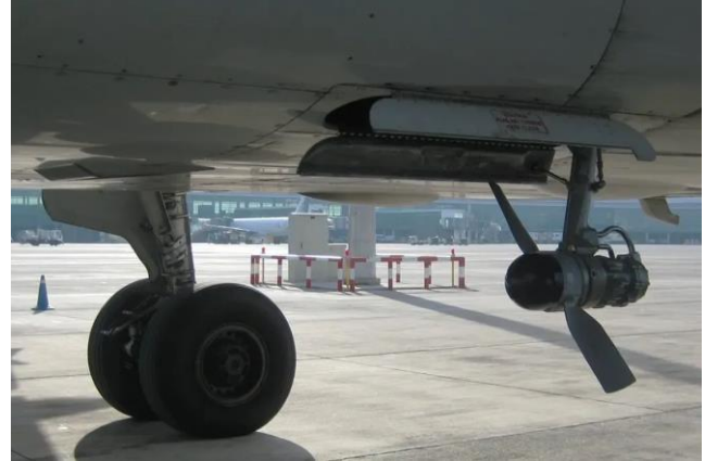
Figure 2. RAT deployed in a grounded aircraft [3].
