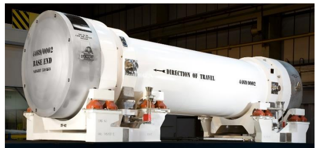
Figure 1. M4/12 Transport package, used to transport Mixed Oxide (MOX) fuels
