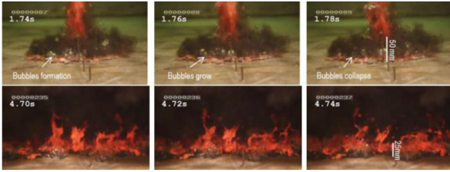
Figure 3: Melt jet and melt spreading with the formation of the premixed layer in the PULiMS-E4 experiment [8].
