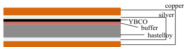
Figure 4. General stacking structure of YBCO HTS tape [16]
