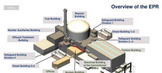
Figure 2. EPR shows a strict application of the basic concept of safety in NPP [8].
