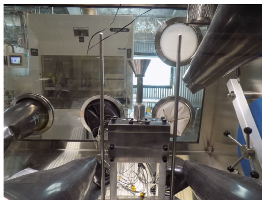
Figure 6. In-process capsule mounting, funnel and salt loading, and rails used for capsule end cap pressing.
